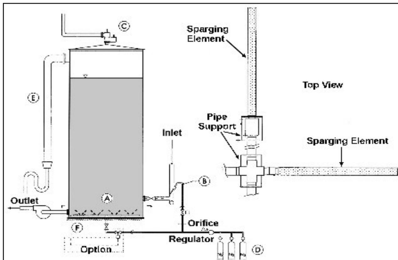
**Figure 1. A Storage Tank Nitrogen System and Sparging Elements**
